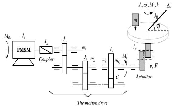
**Fig 1: Dynamic diagram showing the relationships of the elements in the mechanical part of an electric drive system**
