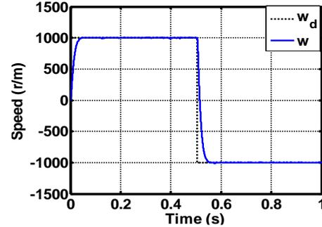
Fig 8: The set speed  $\omega_d$  and actual speed  $\omega$  of case 1
