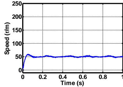
Fig 15: The set speed  $\omega_d$  and actual motor speed  $\omega$  in case 3
