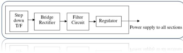
Figure 2. Block Diagram at the Receiver Section
