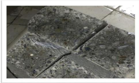
Fig. 8 Penetration level in the second batch of samples
