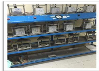
Fig. 6 Water permeability apparatus
