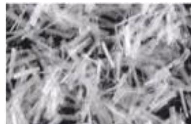
**Fig. 1 Microscopic view of Weber. ad M synthetic fibers**
