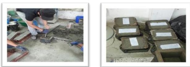
Fig. 2 Casting the samples
