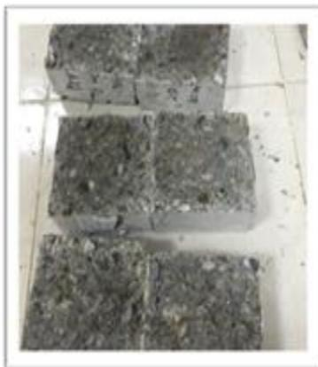
Fig. 7 Samples cut in half to check water penetration
