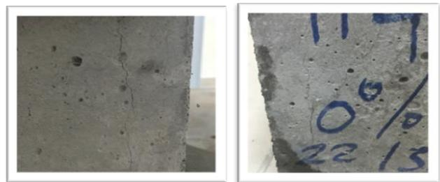
Fig. 3 Cracks formed on the samples
