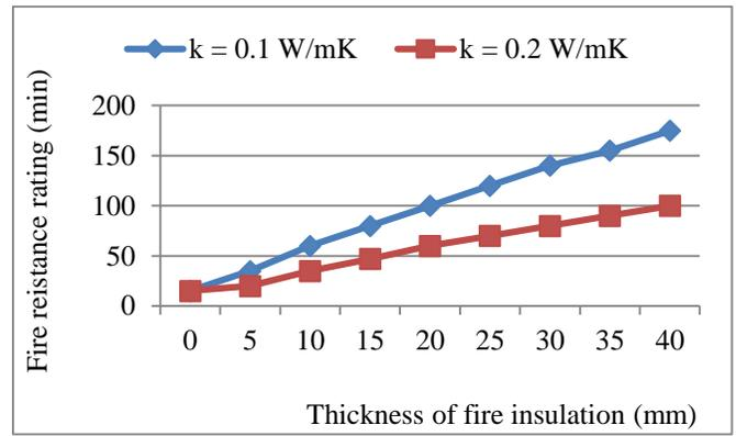
Fig. 2 Effect of insulation thermal conductivity on fire resistance rating of the steel beam
