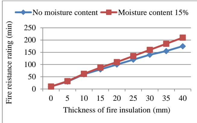
Fig. 3 Effect of insulation moisture content on fire resistance rating of the steel beam
