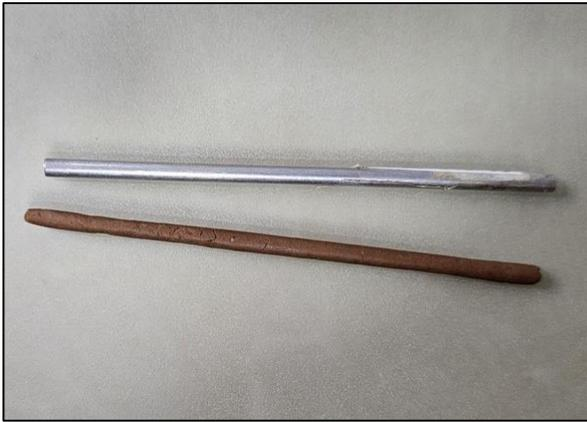
Fig. 10 Plastic limit test
