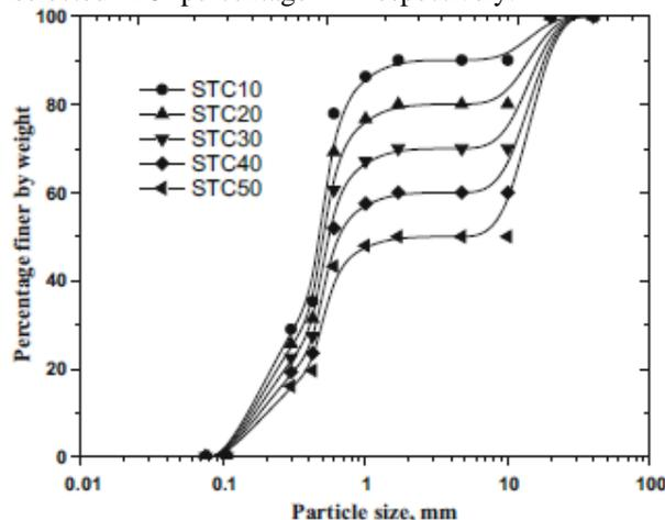
Figure 2 (Grain size distribution of San-Tyre Mixtures)
