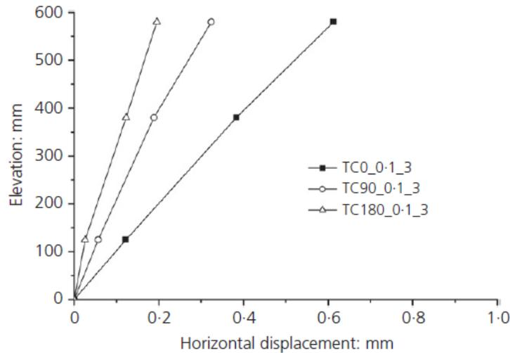
(Fig. No.5 Effect of compressible inclusion on wall displacement for 0.1g\_3Hz)
