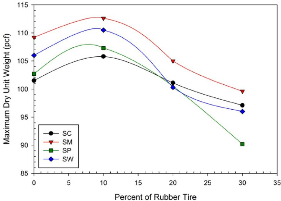
(Figure No.8 Change in Maximum Dry Unit Weight of soil with Different proportion of Rubber)
