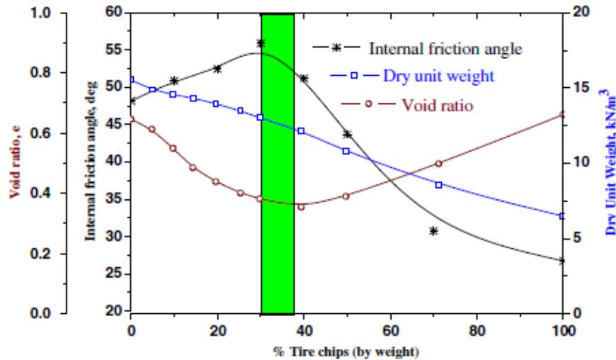
(Fig No.7 Internal friction angle, dry unit weight and void ratio profile with % TC)
