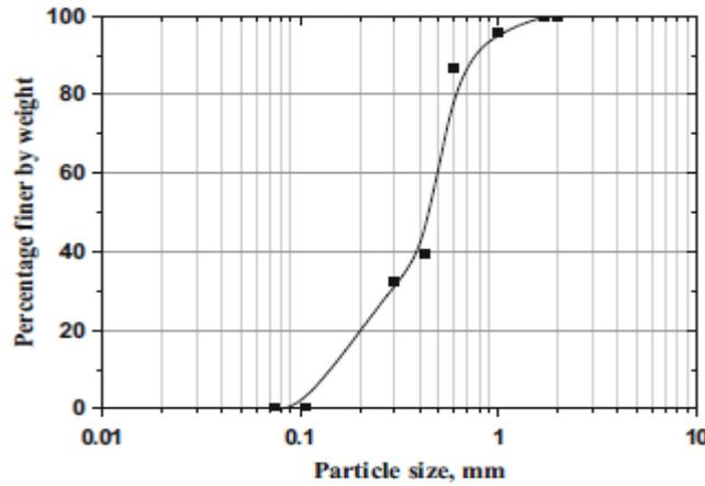
Figure 1.(Grain size distribution of the sand)
