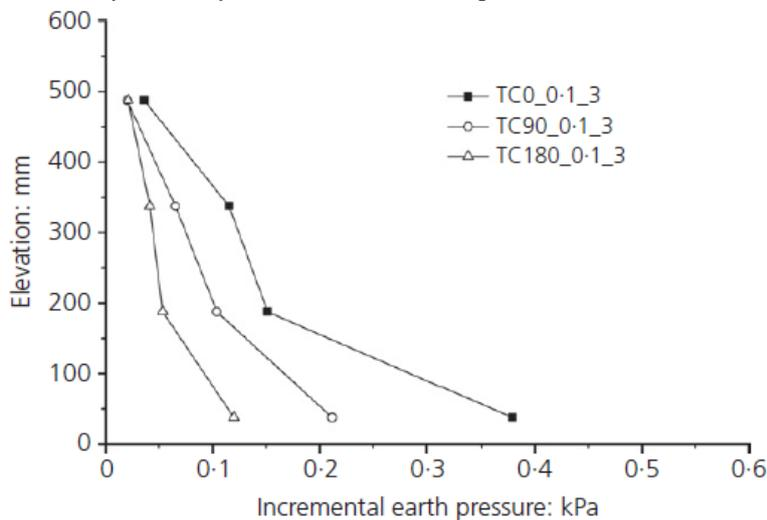
(Fig. No.6 Effect of compressible inclusion on incremental earth pressure for 0.1g\_3Hz)
