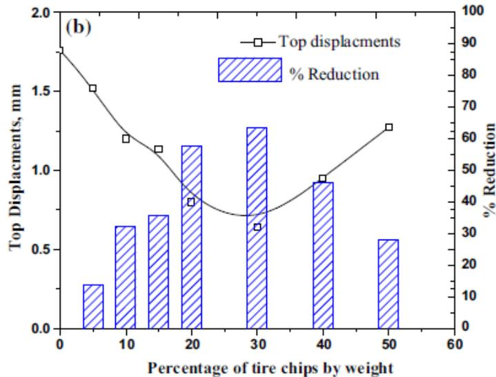
(Fig No.3 Displacement profile with different STC mixtures)
