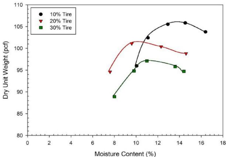
(Figure No. 11 Proctor Compaction Curve for various mixtures of shredded tyres with clayey sand)
