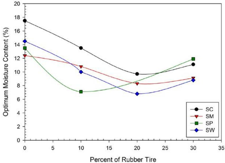
(Figure No.10 Change in OMC of soil with Different proportion of Rubber)
