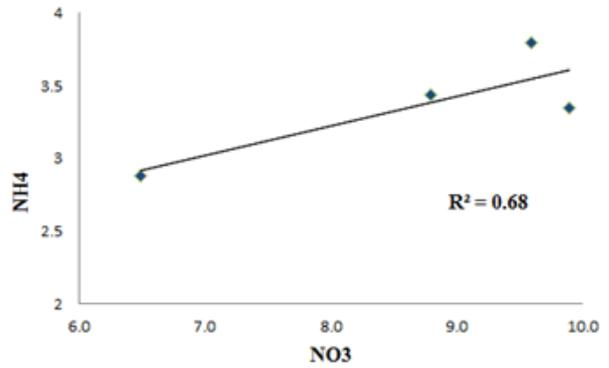
**Fig. 3. Linear regression of the  $\text{NH}_4^+$  and  $\text{NO}_3^-$  in Baqura rainwater samples.**
