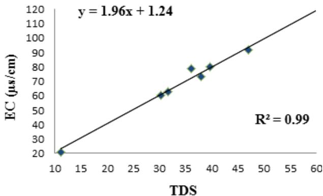
Fig.5. Linear regression of the average EC and TDS values in rainwater samples of the seven stations.
